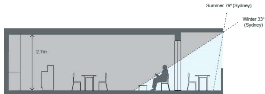
Figure 4A.2 Shading devices on balconies should shade summer sun and allow winter sun access to living areas
