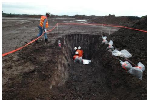
Figure 2. Waste rock sampling activities at Pit J
