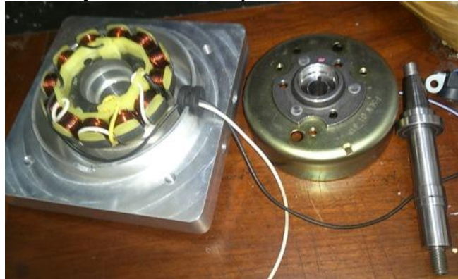
Figure 3 Generator component manufacture
