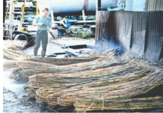
Gambar 5. Proses penggosokan dan pencucian rotan (Sumber, Transfer of Technology Model, Rattan Furniture Making Unit, International Network for Bamboo and Rattan)
