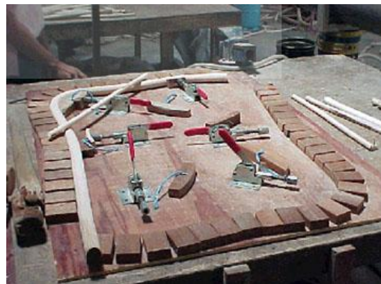
Gambar 11. Proses Pelengkungan Rotan (Sumber, Transfer of Technology Model, Rattan Furniture Making Unit, International Network for Bamboo and Rattan)
