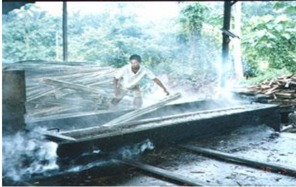
Gambar 4. Proses penggorengan rotan (Sumber, Transfer of Technology Model, Rattan Furniture Making Unit, International Network for Bamboo and Rattan)
