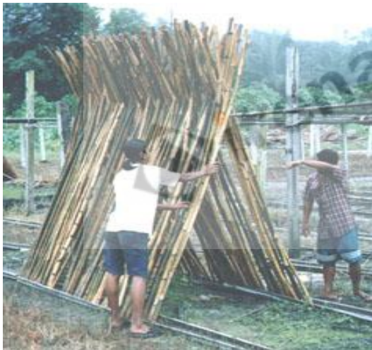
Gambar 6. Proses pengeringan rotan (Sumber, Transfer of Technology Model, Rattan Furniture Making Unit, International Network for Bamboo and Rattan)
