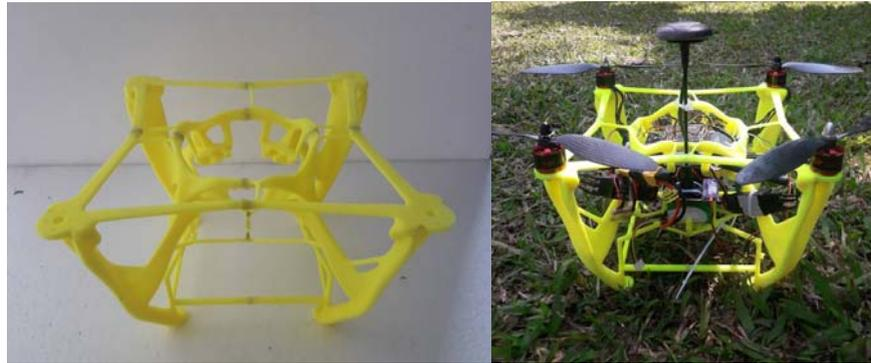
Gambar 2. 3D-printed frame (kiri) dan Autonomous Quadcopter v4.1 with Image Processing System (kanan)
