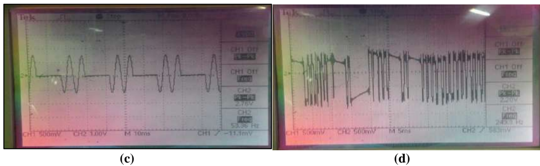
Fig.7 : Output Signal System ASK (a) m-file (b) Simulink (c) Implementation of Modulator output Signal (d) Implementation Signal after Demodulation
