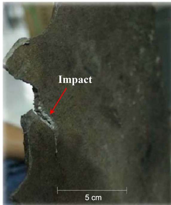
Fig. 10. Notch at the blade leading edge and proceed to crack propagation.
