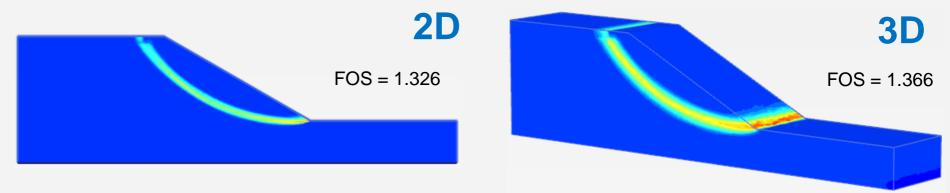
The difference of factor of safety between 2D and 3D model is only 2.93% and the failure mechanism of these methods are similar.
