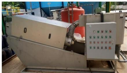
**Gambar 4.11** *Screw Press* di IPL TPA Sarimukti
