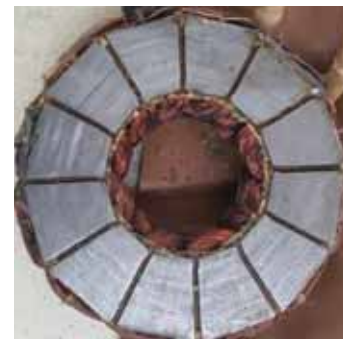
Figure 1 Stator consist of core and armature
