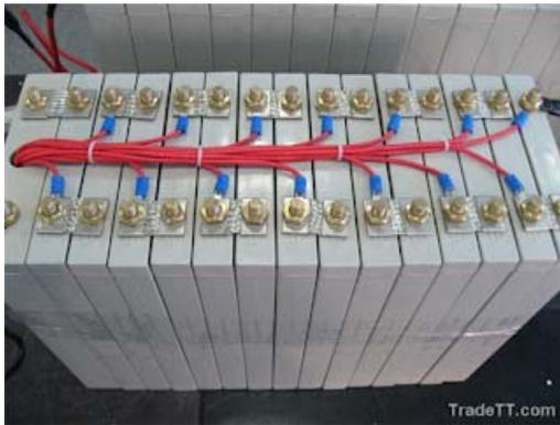
**Gambar 4.35** Rangkaian Baterai *Lithium Prismatic Cell*
