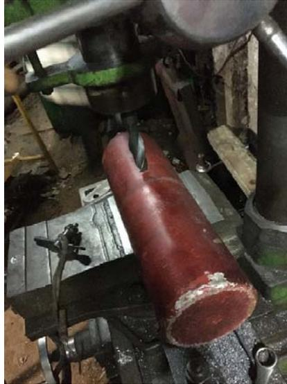
**Gambar 5.7** Proses *Drilling*
