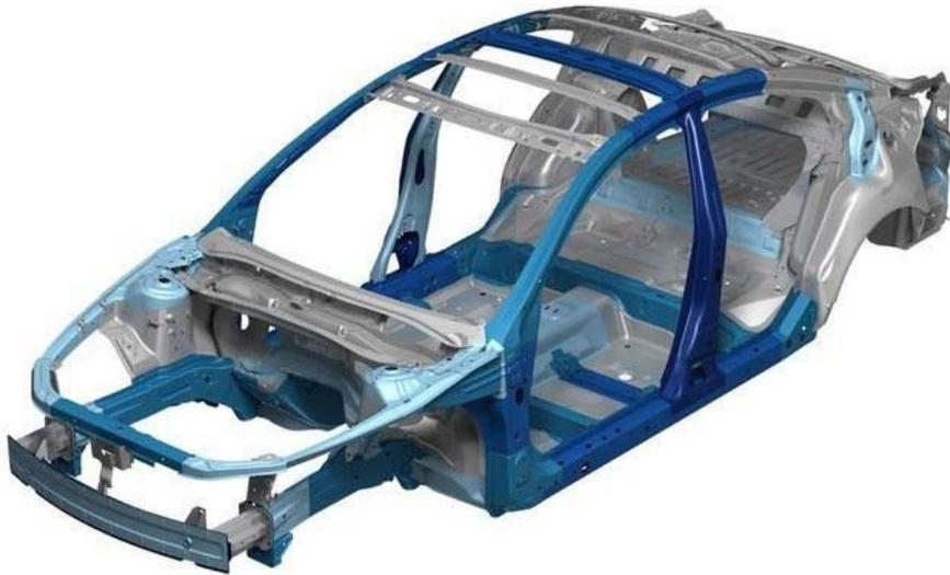
**Gambar 3.4** Rangka *Monocoque*
