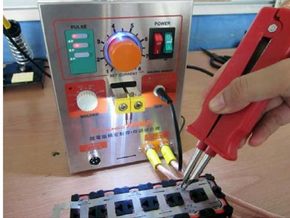
**Gambar 4.33** *Spot Welding Baterai Lithium Cylinder Cell*
