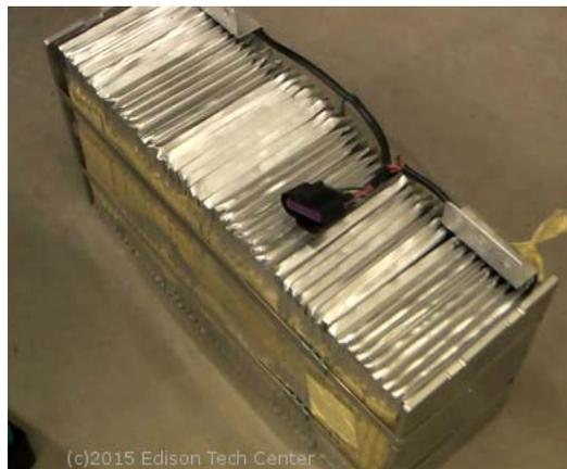
**Gambar 4.34** *Replacement Baterai Lithium Softpack Cell*
