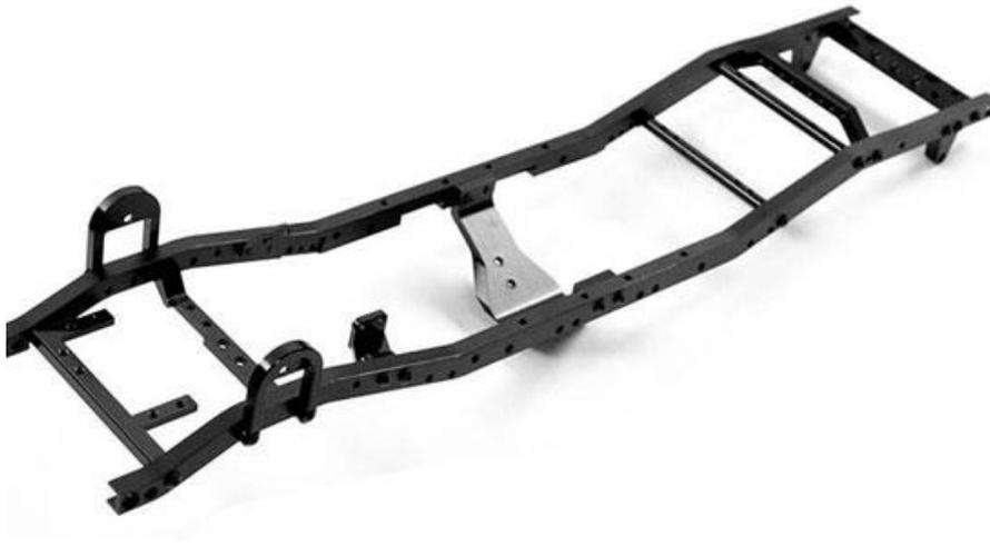
**Gambar 3.2** Rangka *Ladder Frame*
