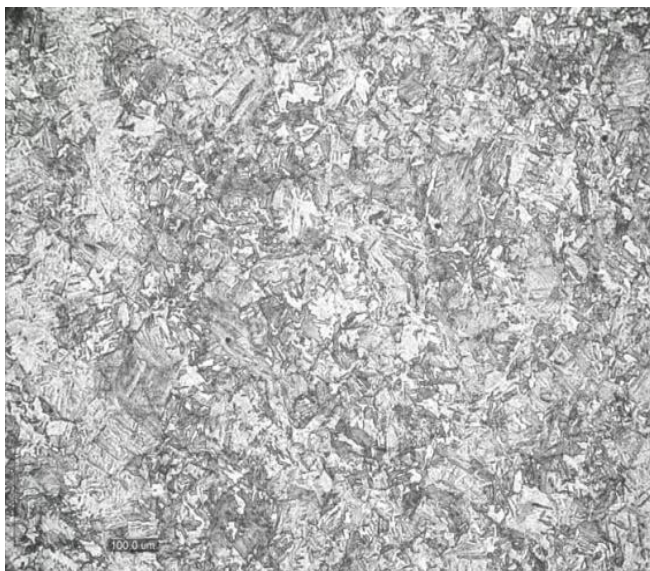
Fig. 4 Microstructure of the broken shackle chain.
