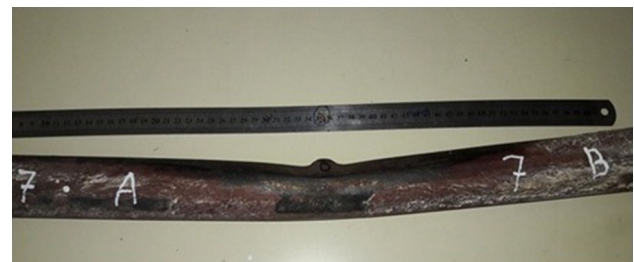
Fig. 5 Failed tube experienced plastic deformation (bowed shaped)
