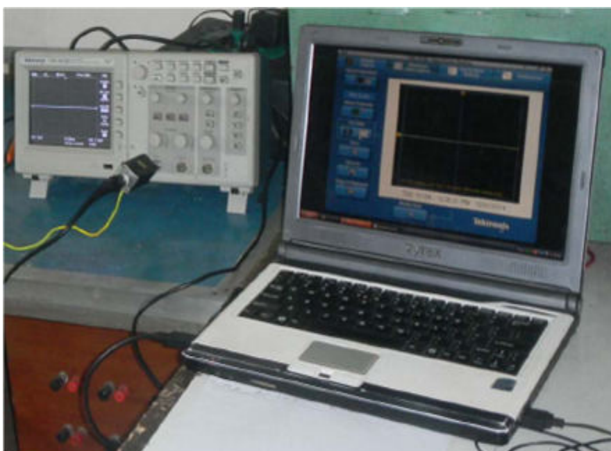
Figure 6. Storage digital oscilloscope and computer for recording and saving measured data
