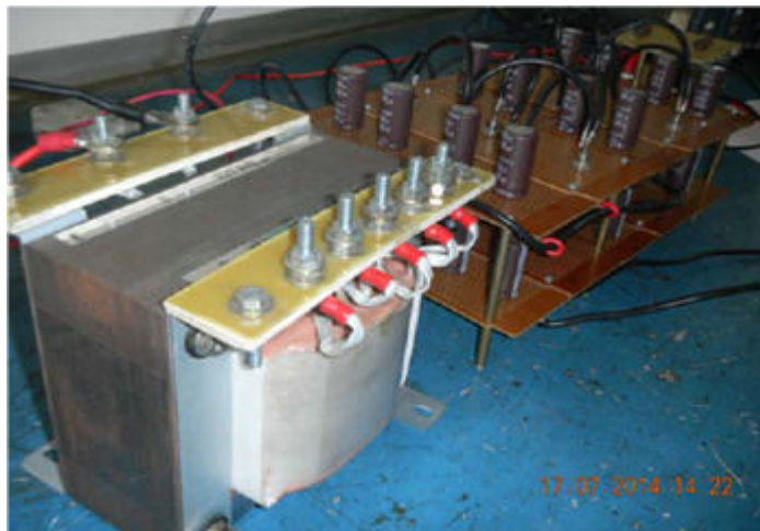
Figure 5. The transformer would be connected to the rectifier and voltage multiplier circuits
