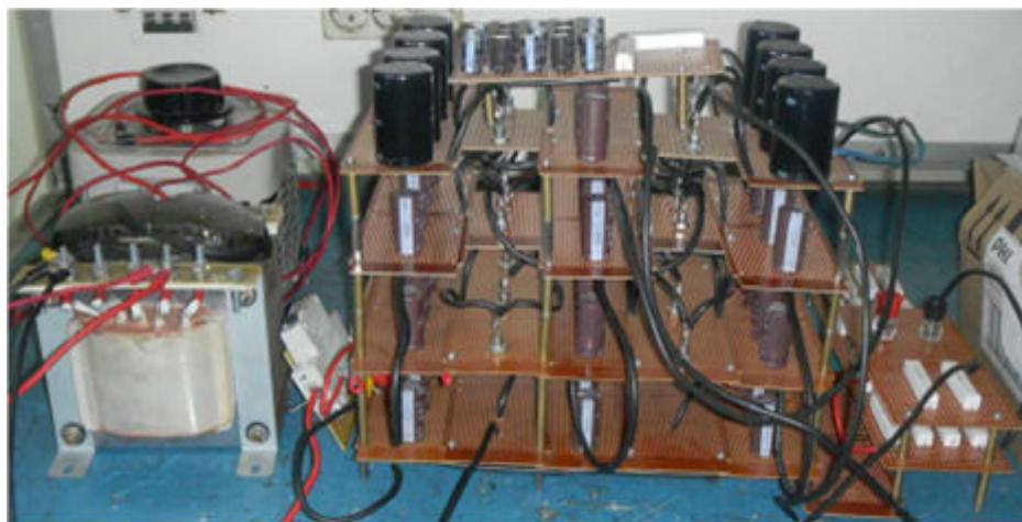
Figure 8. Complete circuit of implemented miniature d.c. high voltage generator
