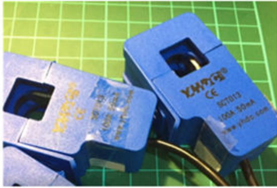
Fig.4: Current transformers for the prototype instrument.
