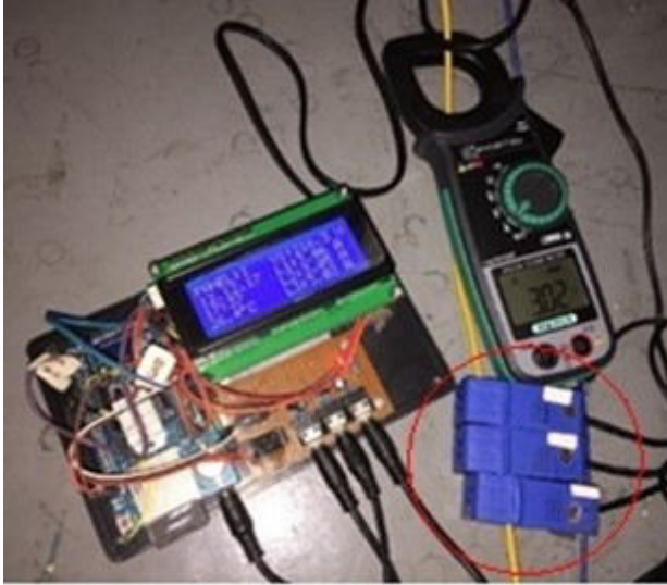
Fig.12: Single-phase current measurement and recording.
