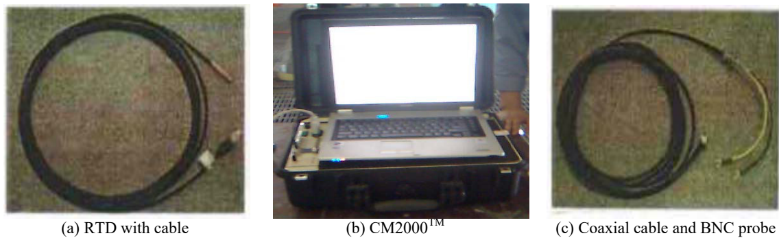
Figure 3. CM2000™ analyzer of partial discharge measurement system and auxiliary cables
