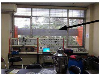
The curtain was fully opened. The illuminance in the room did not comply with the provision.
