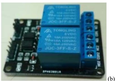
Fig. 4 – a) Circuit diagram and b) two-channel 5-volt dc relay.
