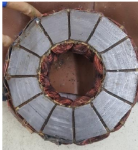
Figure 2. Stator consists of core and armature
