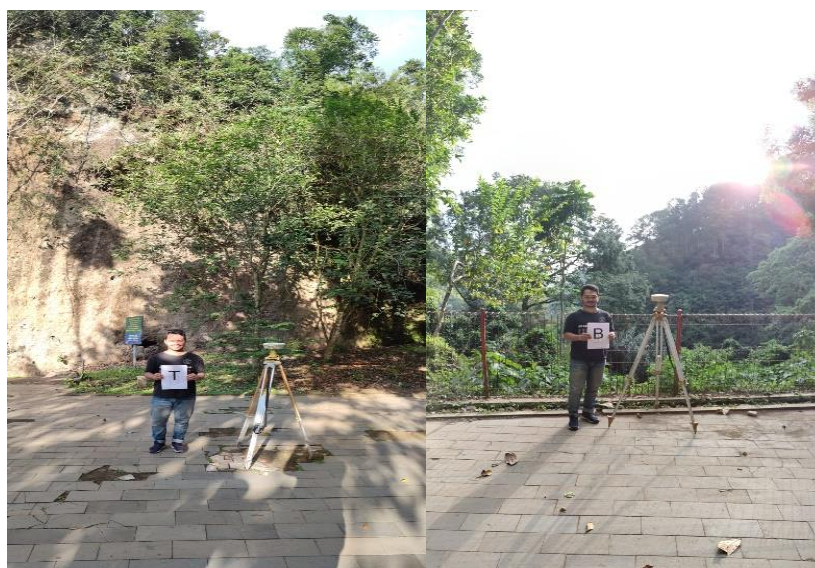
Figure 1. GPS observation in the front area of the Dutch Cave, left side is measurement in BM1 and right side is in BM2.
