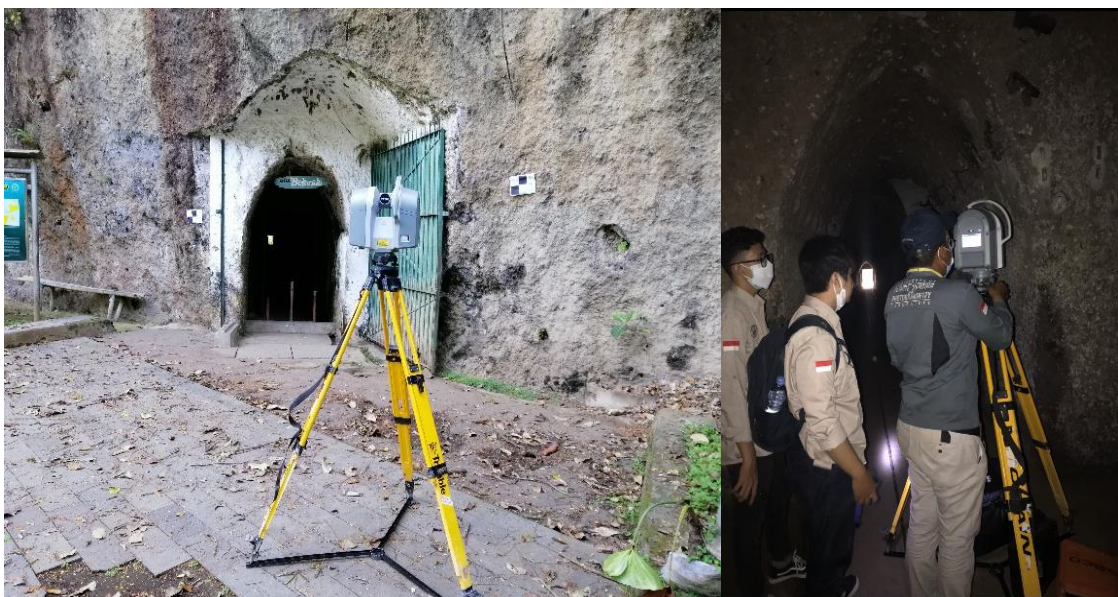
Figure 4. TLS measurement outside Dutch Cave (left) and inside Dutch Cave (right).
