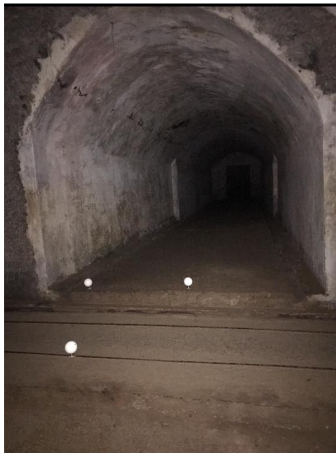
Figure 3. Spherical target position
