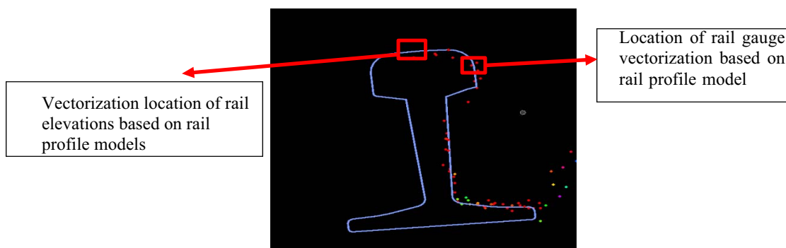
Figure 4. Overlaid rail profile model on point cloud rail
