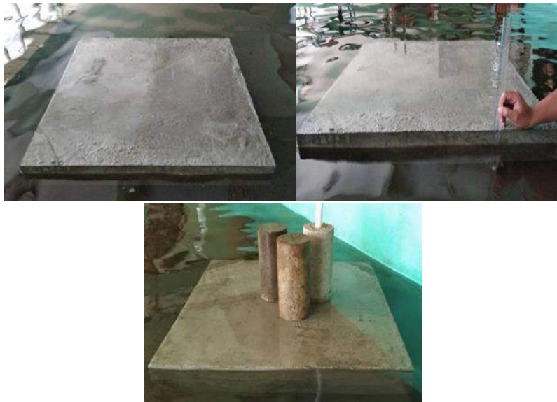
Gambar 9. Setting up benda uji pelat floating concrete
