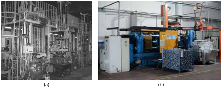
GAMBAR 6.6 Mesin (a) Low Pressure Die Casting (LPDC) dan (b) High Pressure Die Casting (HPDC).
