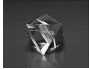
GAMBAR 2.8 Kristal tunggal \text{CaF}_2 . Sumber: www.surfacenet.de/html/picture_crystals.html .
