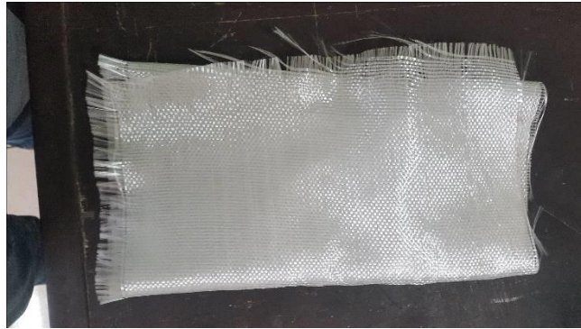
Gambar 2.5 Serat Kaca ( Fiber Glass )
