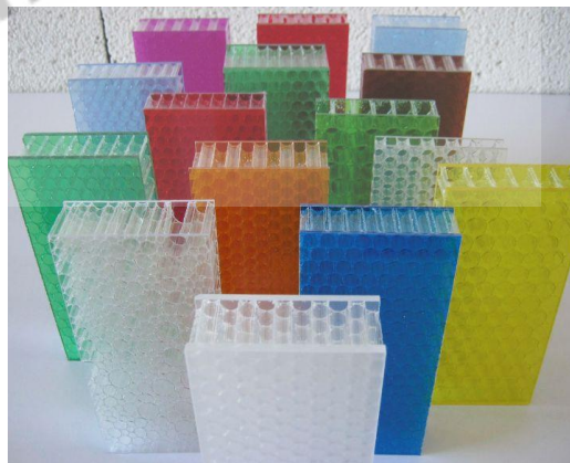
Gambar 2.2 Polycarbonate Honeycomb Panel Sandwich (Tasuns,2017)
