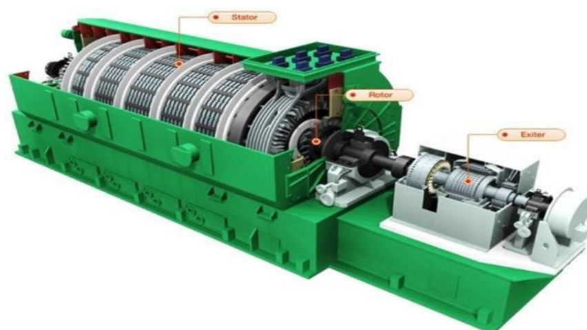
Gambar 2.9 Generator AC ( alternating current ) (Sumber: SuryonoHendry, 2015)
