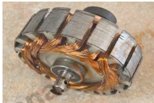
Gambar 2.8 Tampak gulungan generator (Sumber: SuryonoHendry, 2015)
